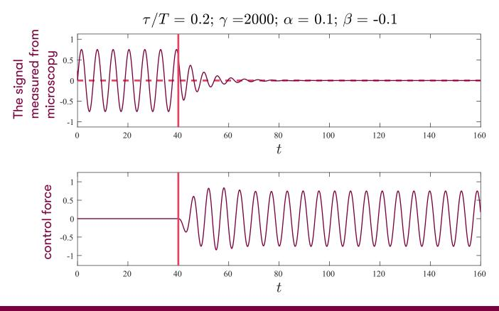
My algorithm is able to detect how the sample should be moved up and down in order to get rid of the first harmonic in the measured signal. Here a numerical demonstration of my algorithm is depicted.
